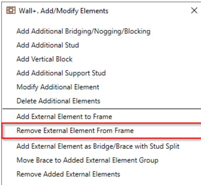
**Remove External Element From Frame** – removes external element from the frame which was previously added to the wall frame.
