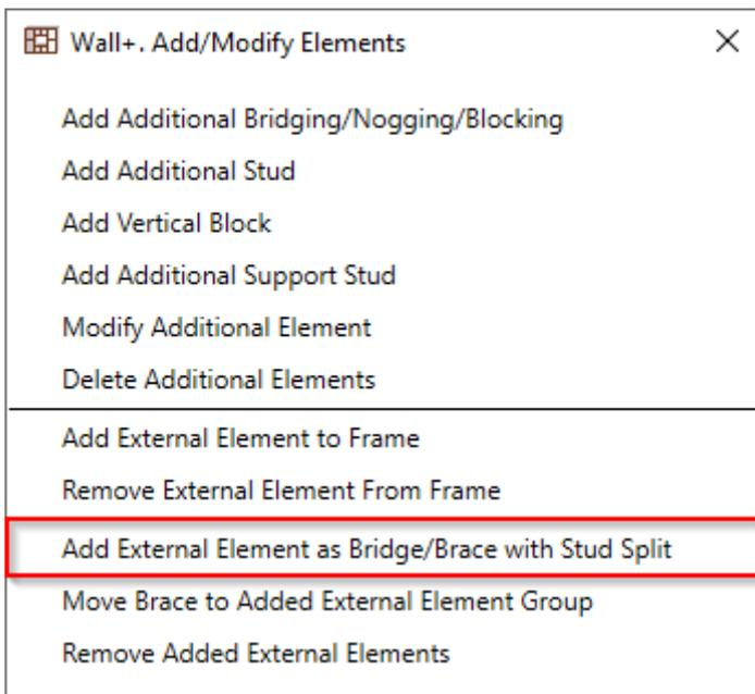
**Add External Element as Bridge/Brace with Stud Split** – adds external element to the wall frame and splits the studs. Select external element or multiple elements and then the wall frame where it should be added.
