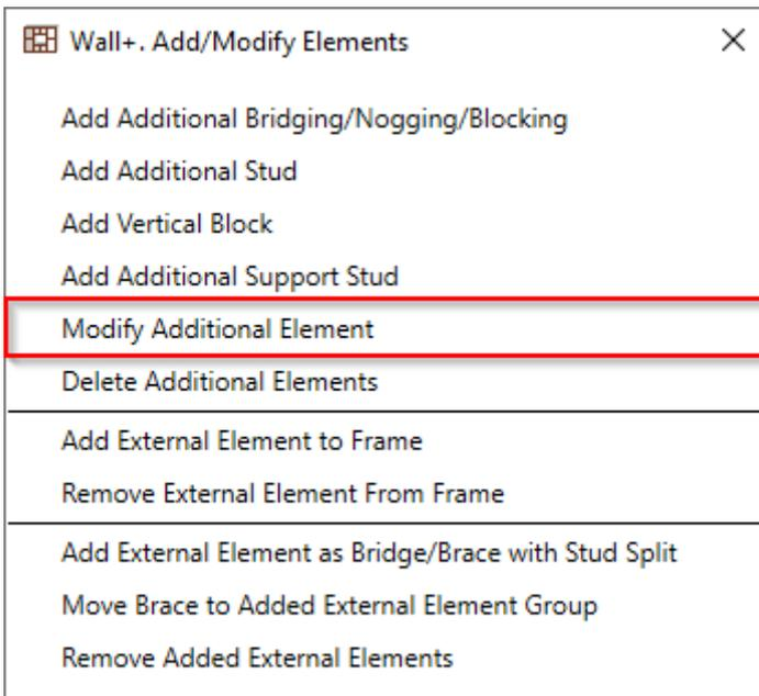
**Modify Additional Element** – modifies selected additional element with custom settings if you need to make unique changes. All settings are the same as were used in the adding process.
