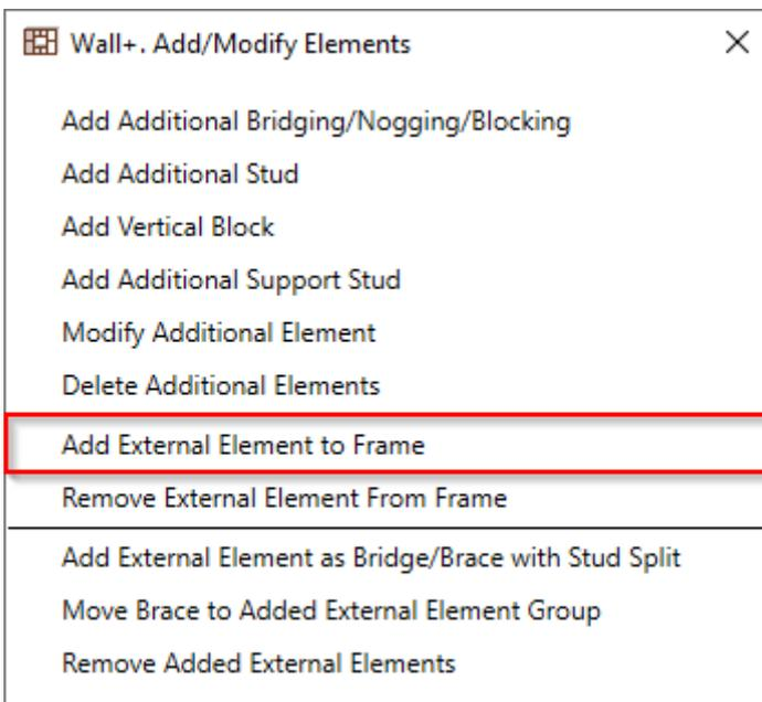
**Add External Element to Frame** – adds external element to the frame. Select external element or multiple elements and then the wall frame where it should be added. Such element will be included while creating assemblies for shop drawings.
