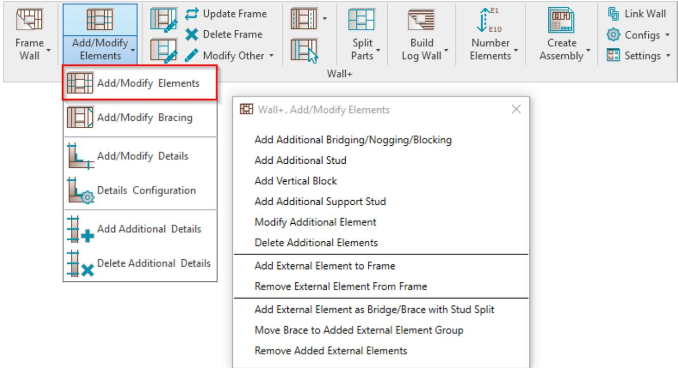
**Add/Modify Elements** – features for adding/modifying additional studs, support studs, bridging/noggin elements, etc.
