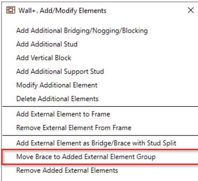
**Move Brace to Added External Element Group** – removes selected brace from frame and splits studs. The braces become external element. Usually used in Floor+.
