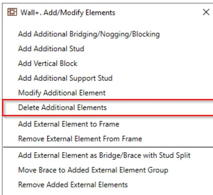
**Delete Additional Elements** – deletes any previously created additional bridging/nogging/blocking, stud, vertical block, or support stud.
