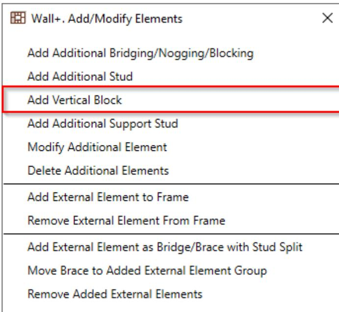
**Add Vertical Block** – adds additional vertical block using studs into selected frame with predefined settings.
