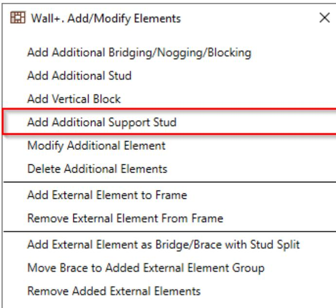
**Add Additional Support Stud** – adds additional support stud between two selected plates.
