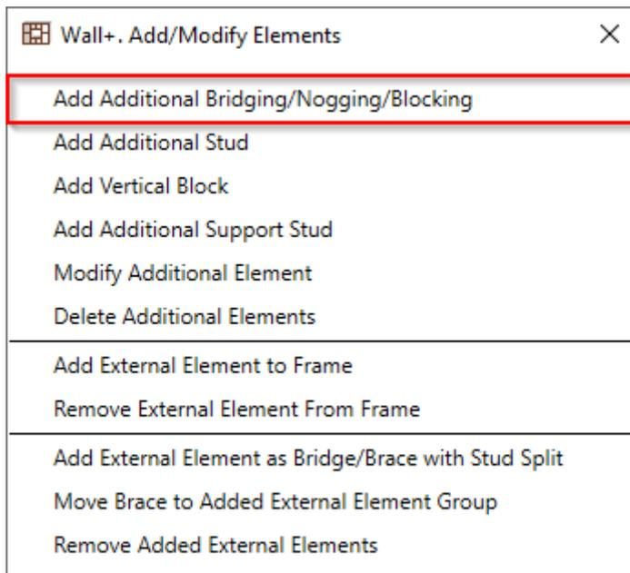
**Add Additional Bridging/Nogging/Blocking** – adds additional bridging/nogging/blocking between selected two studs with predefined settings.
