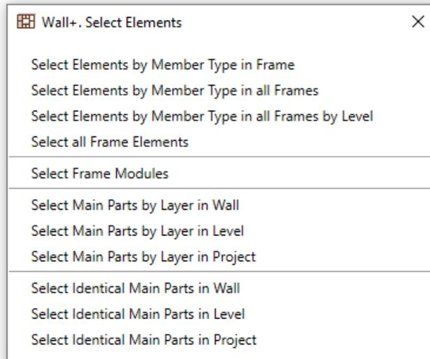
**Select Elements** – features for quickly selecting elements by different rules.
