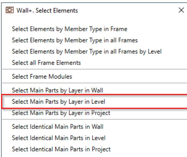
**Select Main Parts by Layer in Level** – selects main parts in the same type of framed walls in the same level.
