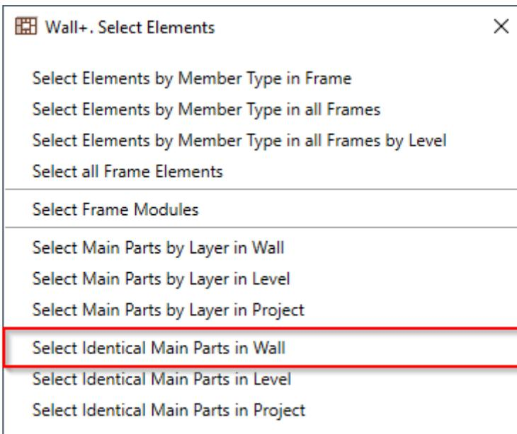
**Select Identical Main Parts in Wall** – selects identical main parts in the framed wall.
