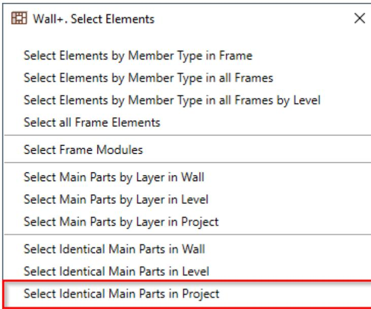
**Select Identical Main Parts in Project** – selects identical main parts of framed walls in the whole project.
