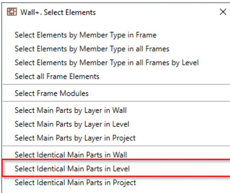
**Select Identical Main Parts in Level** – selects identical main parts of framed walls in the same level.
