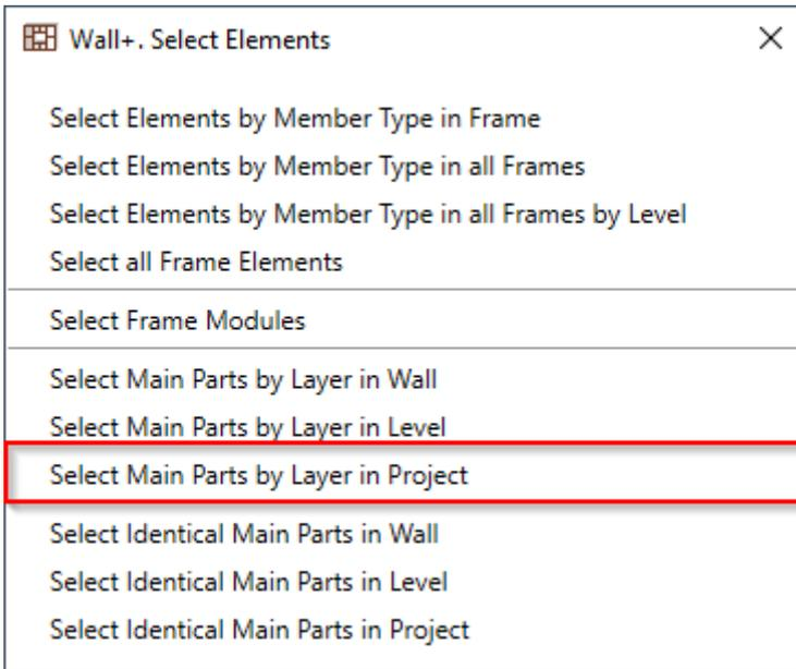
**Select Main Parts by Layer in Project** – selects main parts in the same type of framed walls in the whole project.
