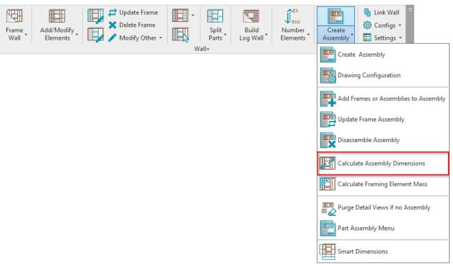
Calculate Assembly Dimensions – calculates assembly dimensions (area, volume, width, depth, length, height) by predefined rules and writes the results in assembly instance parameters (Assembly Area, Assembly Volume, Assembly Width, Assembly Depth, Assembly Length, Assembly Height) for later use in schedules.
