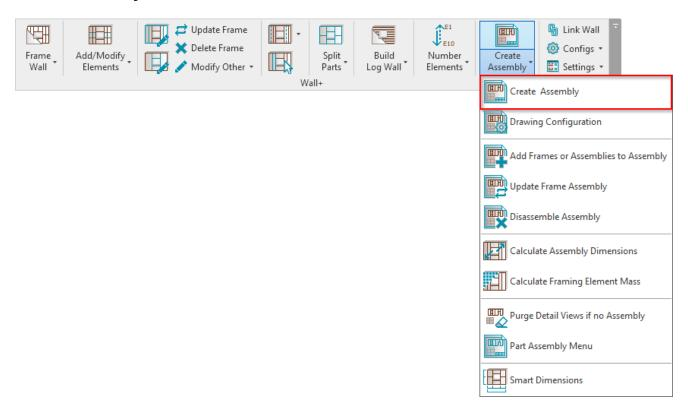
**Create Assembly** – makes shop drawings for selected walls. Select any frame from the wall, and after clicking **Create Assembly**, the software will create shop drawings according to the predefined configuration.
