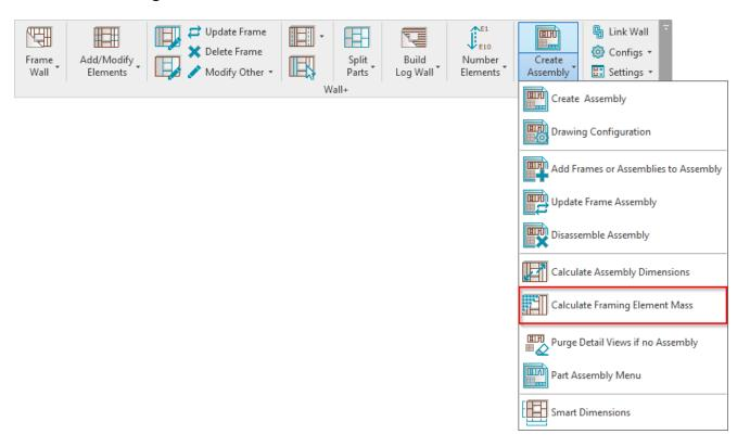
Calculate Framing Element Mass – calculates mass of selected framing elements, and writes result to Framing Member Mass parameter, which you can find in Element Properties → Identity Data.
