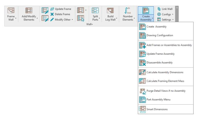
Wall+ will collect all elements from one wall panel and make an assembly with predefined views, add dimensions, add tags, make sheets, and put the views into the sheets.
