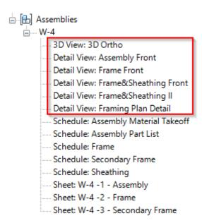
**Create Detail View** – whereas with a simple assembly view you see only the assembly itself – in isolation from other parts with which it interacts – Detail Views lets you see how a given assembly relates to other pieces of the pie, like walls, floors, elevations, grids, etc.
