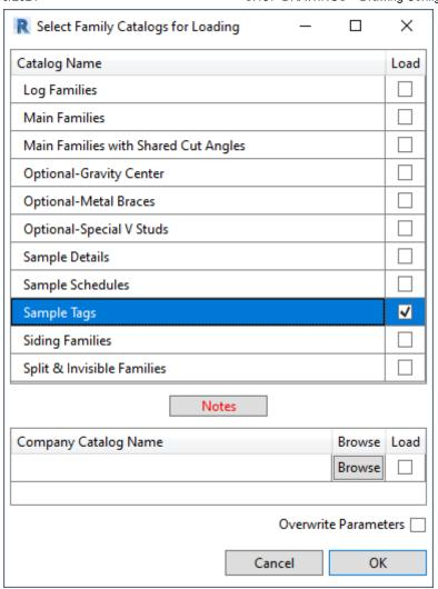
Structural Framing Tag – select a family for tagging all studs and plates in the view.
