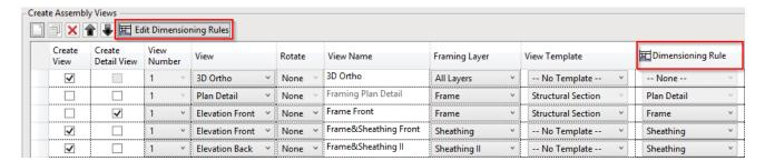
**Dimensioning Rule** – dimensioning rules for the selected view. Dimensioning rules are saved under separate names and can be used for other projects.
