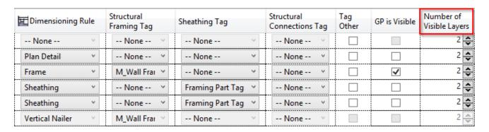
Number of Visible Layers – allows you to add the number of visible layers in the view.
