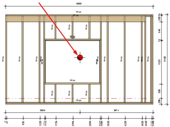
The Gravity Point also can be dimensioned in the assembly view. All dimensioning rules are in **Smart Dimensions**:
