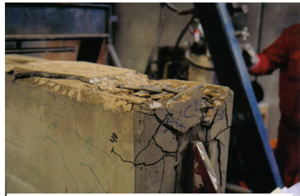
Figure 15. The end of test 3 after brittle failure at R \approx 350 kN.
