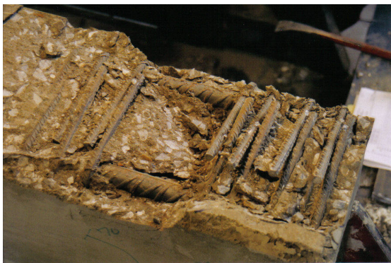
Figure 16. Top of stirrups after brittle failure at R \approx 350 kN.
