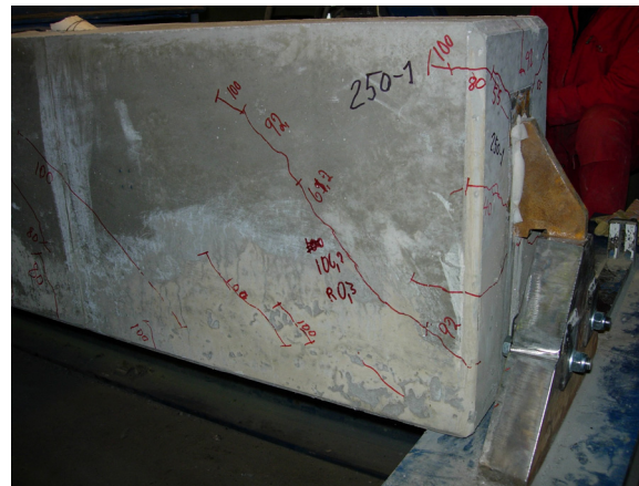
Figure 7. Beam end at R = 438 kN
