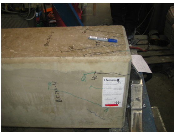
Figure 19. Test 4 at R ≈ 310 kN
