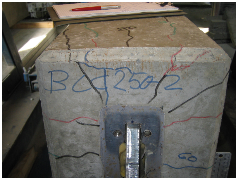
Figure 13. Test 2 at R \approx 370 kN.
