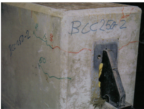
Figure 11. Test 2 at R \approx 210 kN.
