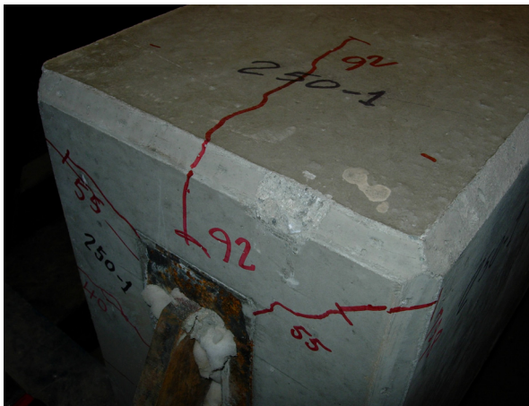
Figure 6. Beam end at R = 380 kN
