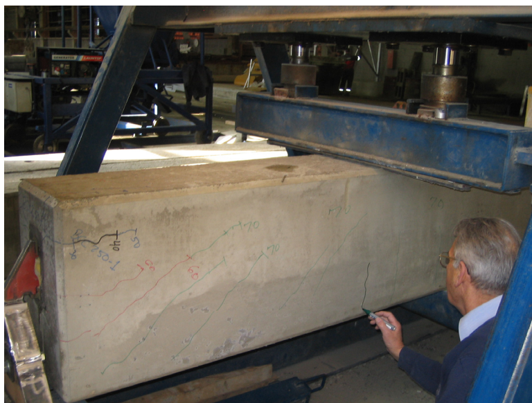
Figure 10. Test 1 at R ≈ 300 kN.
