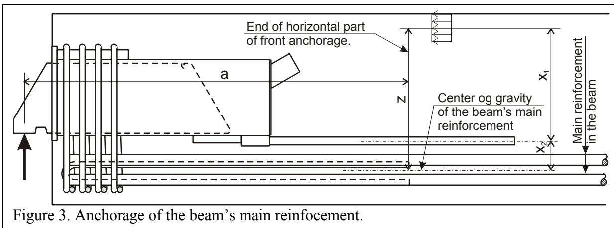
Figure 3. Anchorage of the beam's main reinforcement.
