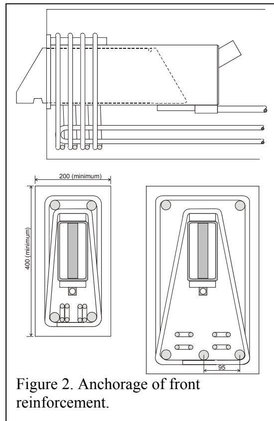
Figure 2. Anchorage of front reinforcement.
