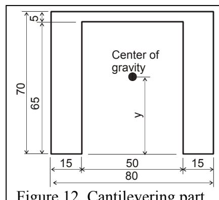
Figure 12. Cantilevering part of top plate.
