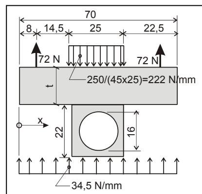
Figure 14. Forces on the bottom plate.
