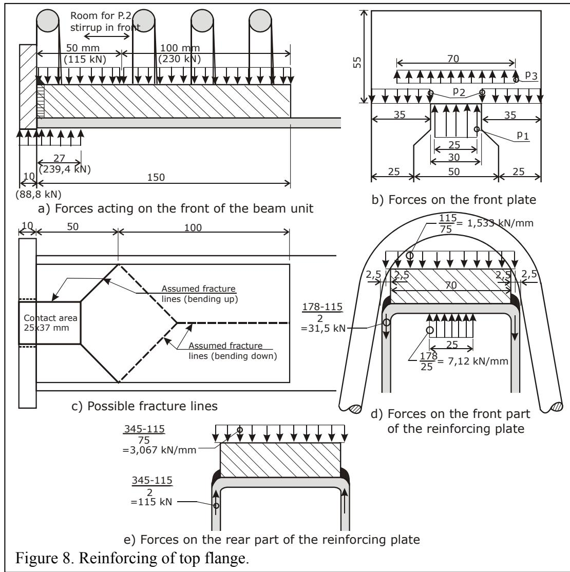
Figure 8. Reinforcing of top flange.
