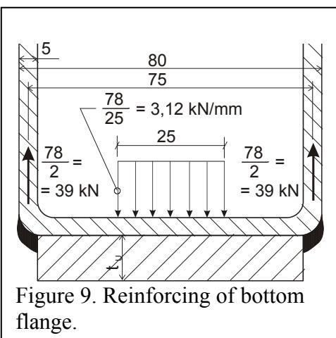
$$\begin{aligned} M &= 39 \cdot 75 / 2 - 3,12 \cdot (25/2)^2 / 2 \\ M &= 1219 \text{ kNm} \\ \text{Req'd. } W &= 1219 / 0,355 = 3433 \text{ mm}^3 \end{aligned}$$
