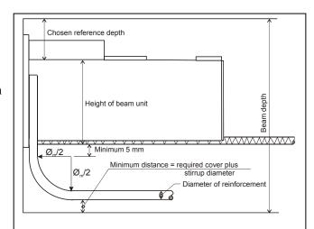
Figure 4. Bending of front reinforcement.
