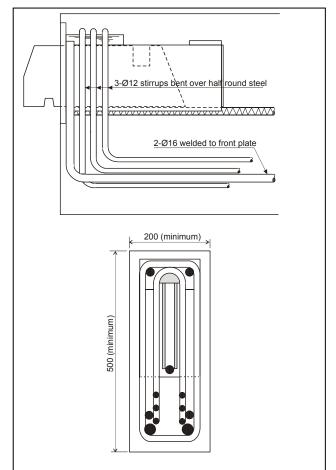
Figure 2. Anchorage of front reinforcement.
