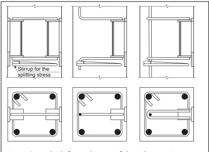
Figure 6. Methods for anchorage of the column unit.
