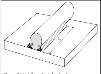
Figure 7. Welding of reinforcing bars.
