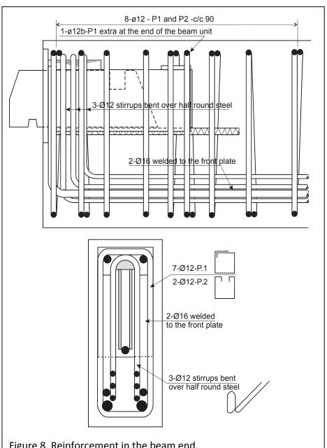
Figure 8. Reinforcement in the beam end.
