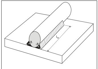
Figure 7. Welding of reinforcing bars.
