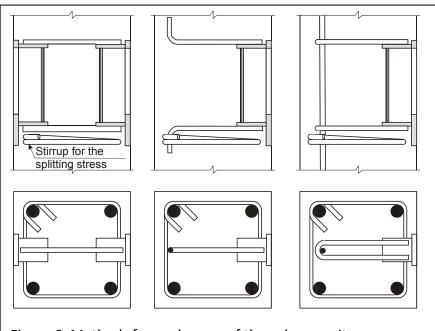
Figure 6. Methods for anchorage of the column unit.
