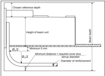
Figure 4. Bending of front reinforcement.
