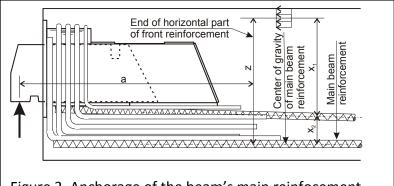
Figure 3. Anchorage of the beam's main reinfocement.
