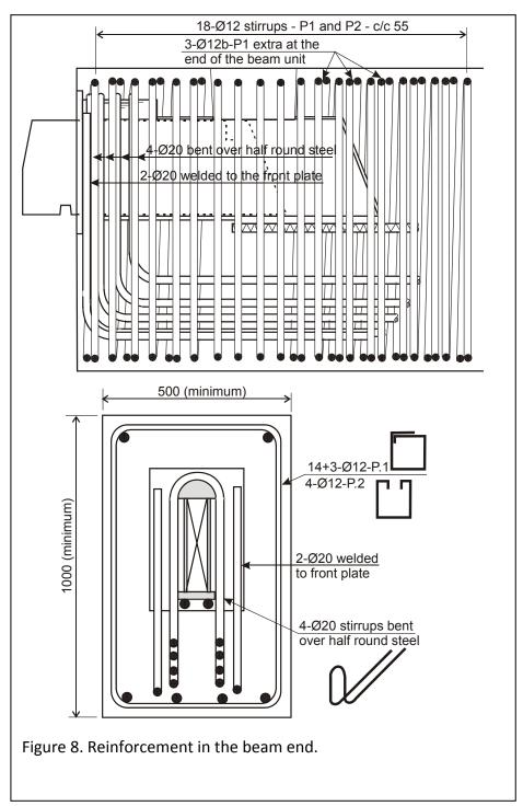
At the end of the front anchorage it must be checked that the beam's main reinforcement has sufficient anchorage. See clause 2.2.4.
