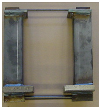
Picture shows at BCC450 column unit. Two sided unit
