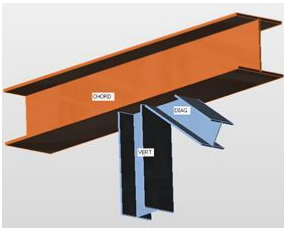
Figure 9: Geometry of joint with open cross-sections
