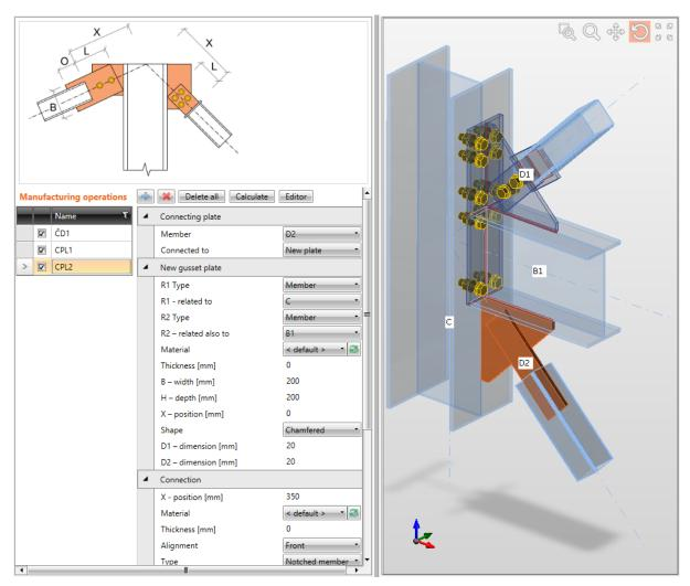
Connection of diagonals D1 and D2 (rectangular hollow sections) to the frame knee.
