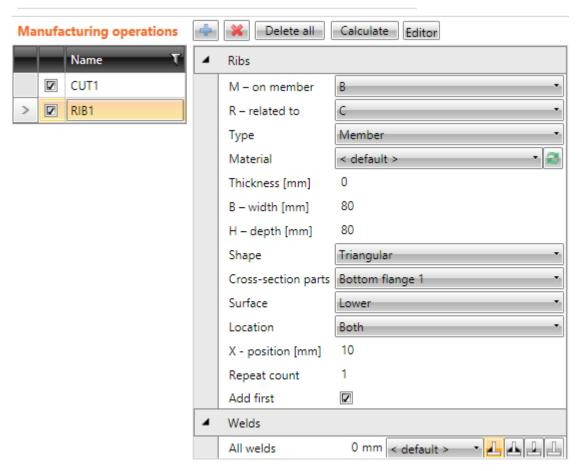
Properties of manufacturing operation **Rib**:
