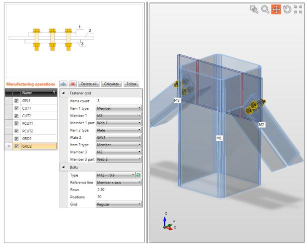
Manufacturing operation General plate is applied on member M1. The operation creates plate at the end of member. Manufacturing operations Plate cut are applied on flanges of member M1 to create notches for the plate. The plate is welded to flanges in notches.
