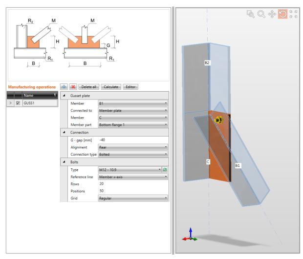
Bolted connection of diagonal to the cross-section part.
