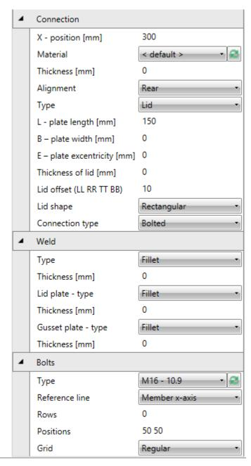
Properties of manufacturing operation Connecting plate:
