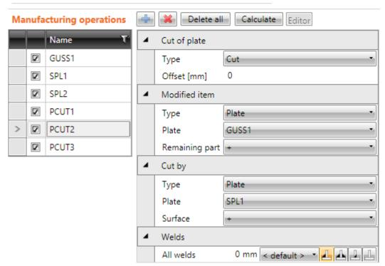
Properties of manufacturing operation **Plate cut**:
