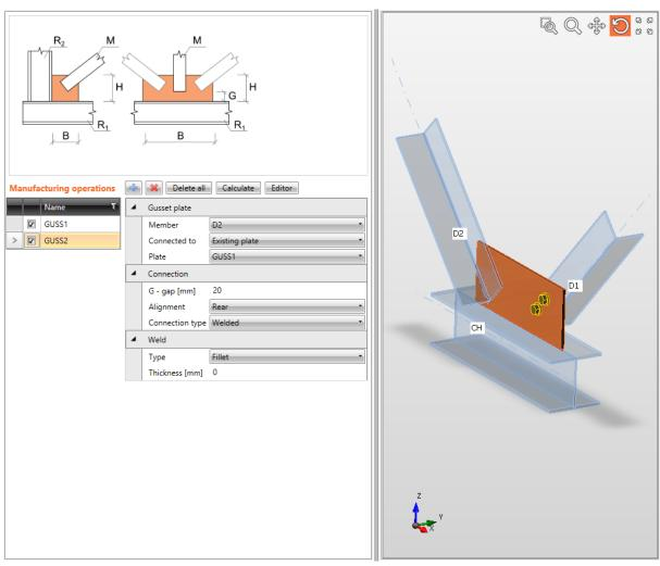
Welded connection of bracing diagonal to an existing gusset plate.
