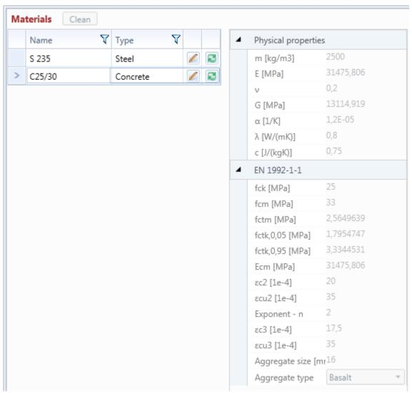
All materials, which are assigned to cross-sections in the project, are listed in the **Materials** table.
