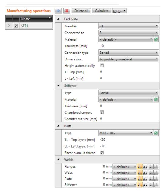
Properties of manufacturing operation Shifted end plate:
