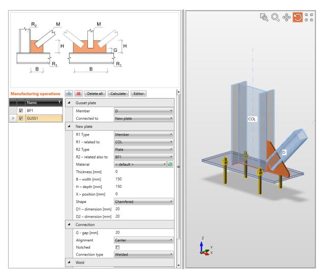
Bolted connection of bracing diagonal to the base plate using gusset plate.
