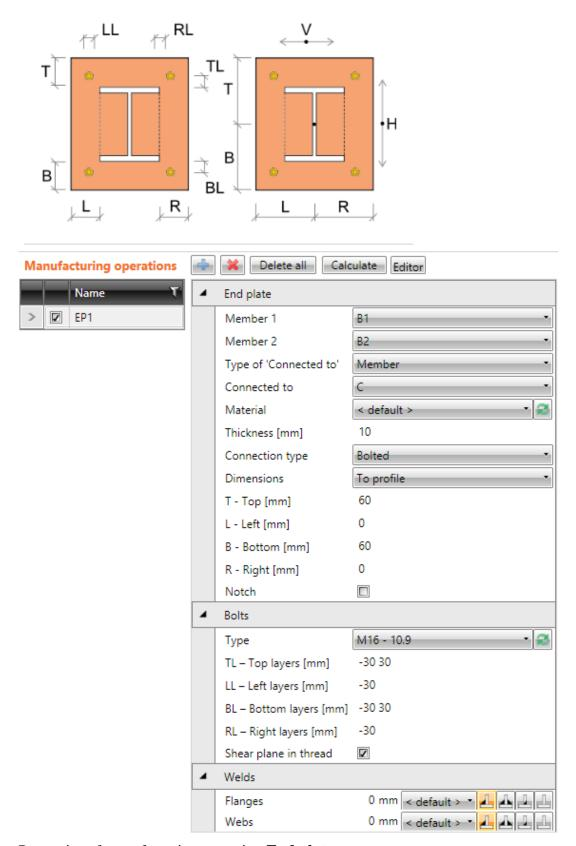
Properties of manufacturing operation End plate:
