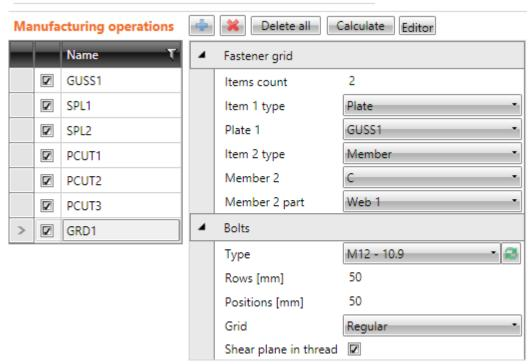
Properties of manufacturing operation Fasteners grid:
