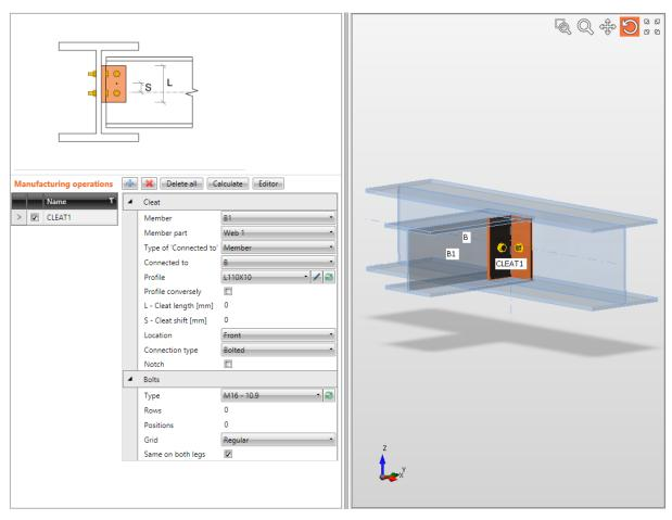
Manufacturing operation Cleat is applied on member B1. The cleat is applied on both sided of web of member B1 and it is connected to the web of beam B using bolts assembly.
