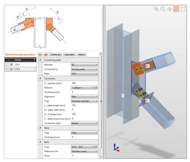
Connection of bracing diagonal B2 (rectangular hollow section) to an existing connecting plate.
