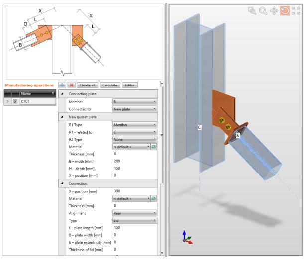
Connection of bracing diagonal B (rectangular hollow section) to a new connecting plate.
