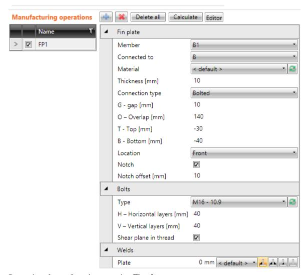
Properties of manufacturing operation **Fin plate**:
