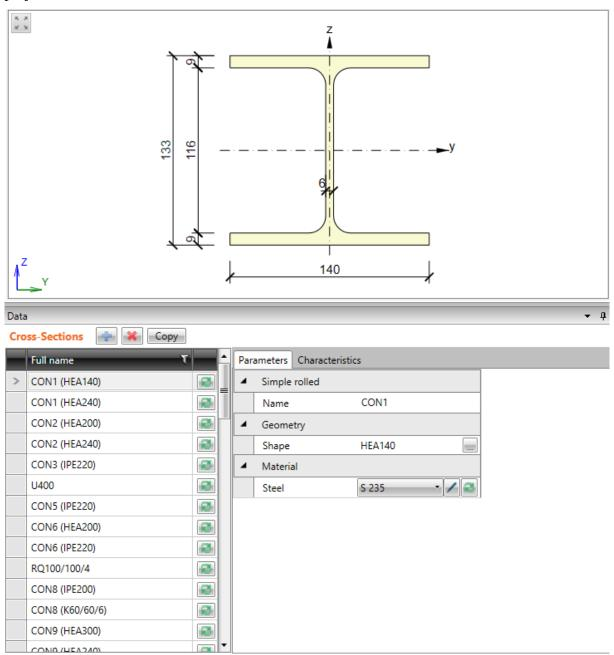
Click **Copy** above the table of cross-sections to copy an existing cross-section.
