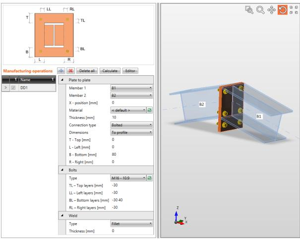
Bolted plate to plate connection.
