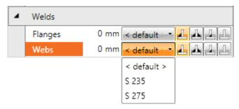
**Each** modifiable weld (group of welds) in the manufacturing operation is represented by one row in welds table. Following properties can be set for individual weld:
