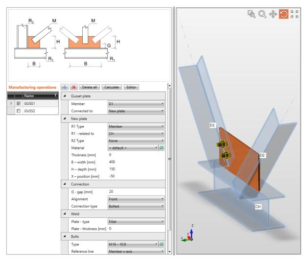
Bolted connection of bracing diagonal to a new gusset plate.
