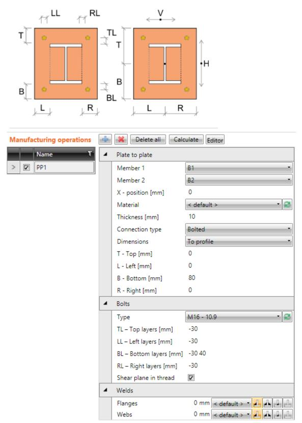
Properties of manufacturing operation Plate to plate:
