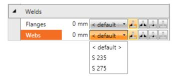
**Each** modifiable weld (group of welds) in the manufacturing operation is represented by one row in welds table. Following properties can be set for individual weld:
