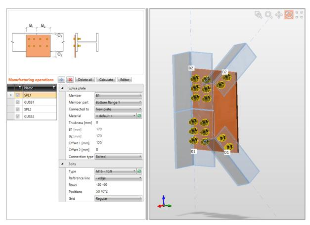
Combined operations Splice and Gusset plate to connect two beams (angle sections) and to connect diagonals (also angle sections).
