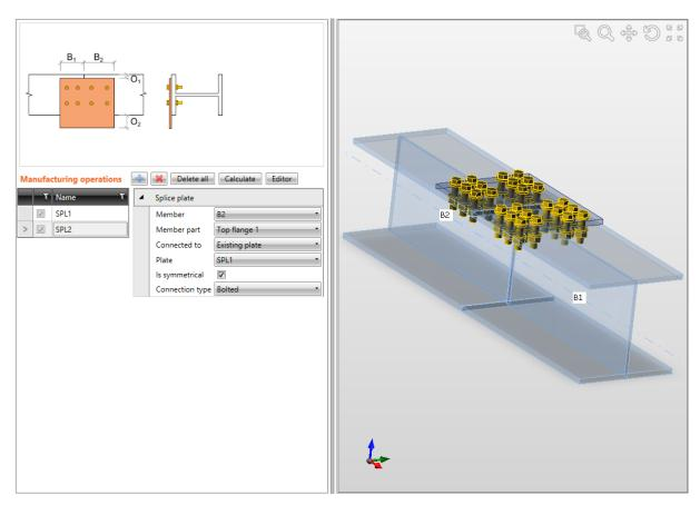
Connecting beam flange to existing splice.
