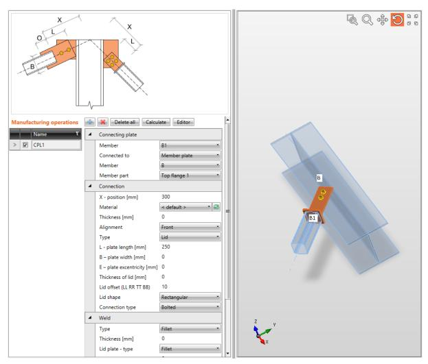
Connection of diagonal to a cross-section part.
