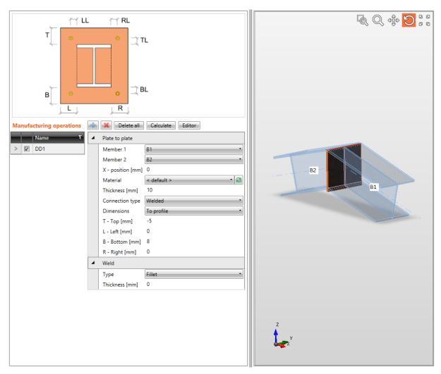
Welded plate to plate connection.
