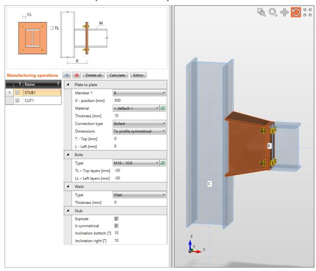
Stub bolted on beam and welded on column.
