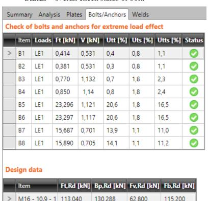
Columns in the table **Check of bolts and anchors** (when checking anchors):
