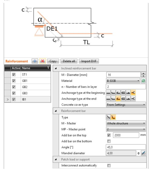
Properties group **Inclined reinforcement bar**:
