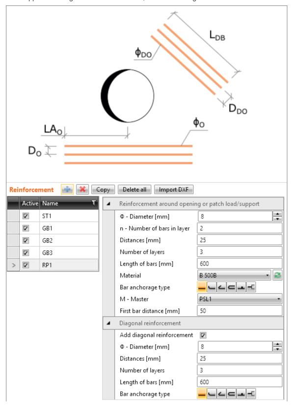
Properties group Reinforcement around opening or patch/load support:
