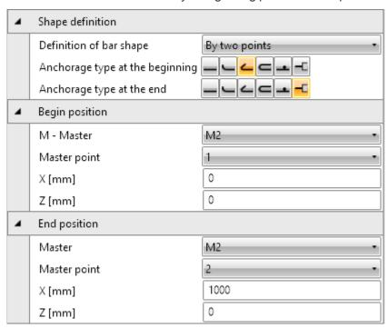
Properties groups **Begin position** and **End position** – definition of beginning/end point position for input mode **By two points**:
