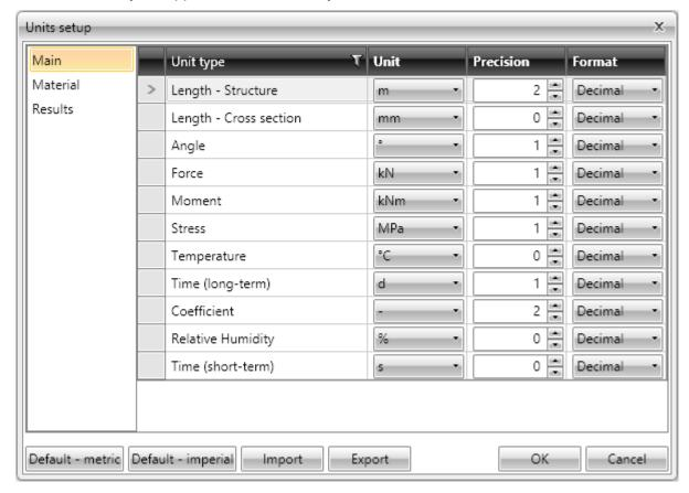
Magnitudes, for which the units can be set, are grouped into categories Main, Material and Results. The categories are displayed in the column on the left of the dialog. For the selected category the table of corresponding magnitudes is displayed. For each magnitude, which is listed in column **Unit type**, one of the available units can be set in the column **Unit**.
