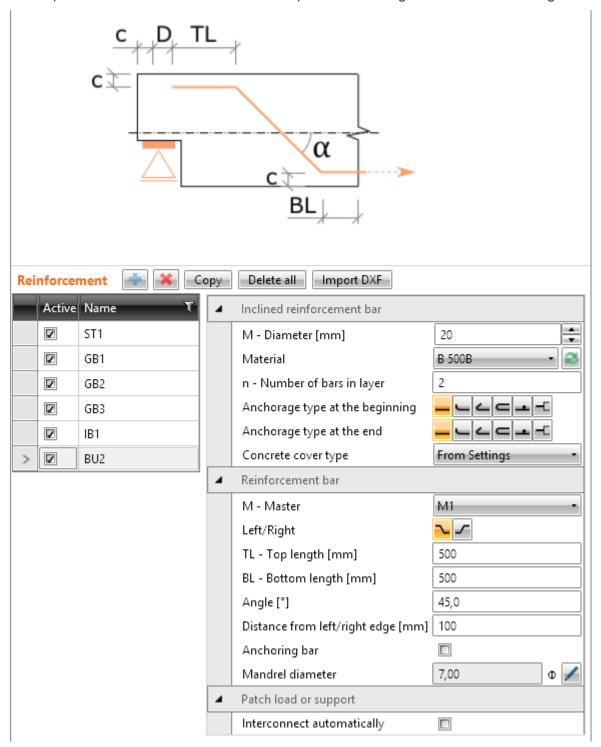
Properties group Inclined reinforcement bar:
