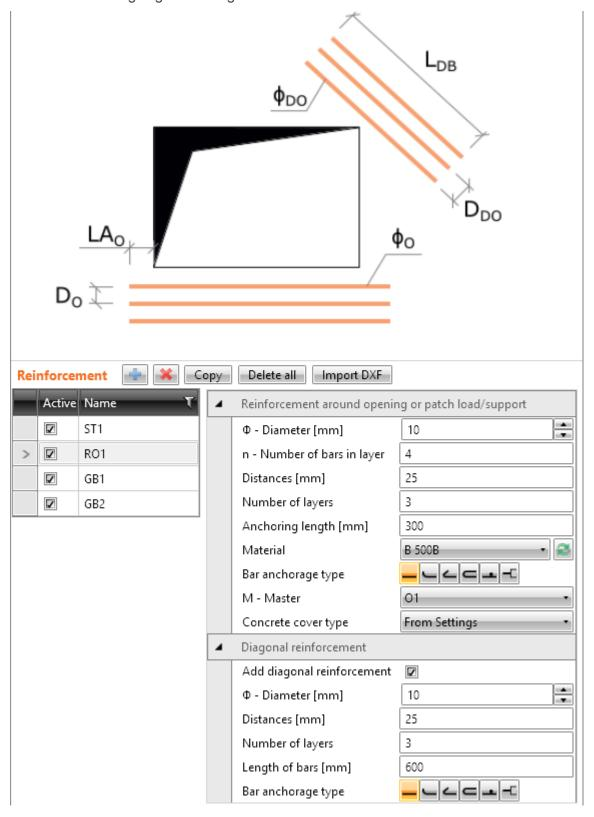
Properties group Reinforcement around opening or patch/load support:
