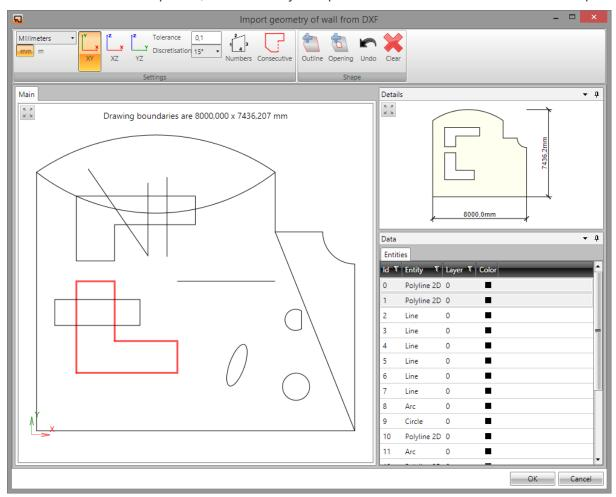
The content of imported DXF file is displayed in the dialog **Import geometry of wall from DXF**.
