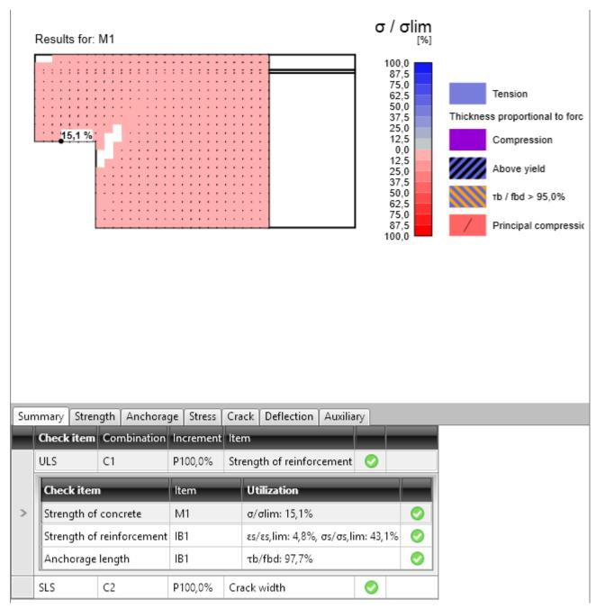
Summary check results of concrete and reinforcement for the selected or extreme load case can be evaluated on the tab **Summary**.
