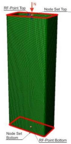
Comparison of the Buckling Resistance of SHS and RHS Profiles
