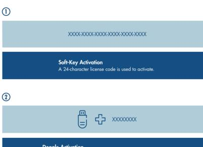
**Dongle Activation** A dongle and an 8-character license code are used to activate.
