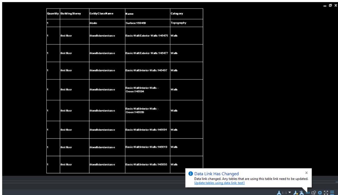
*Figure 3. Notification balloon pops up when the data link has changed*
