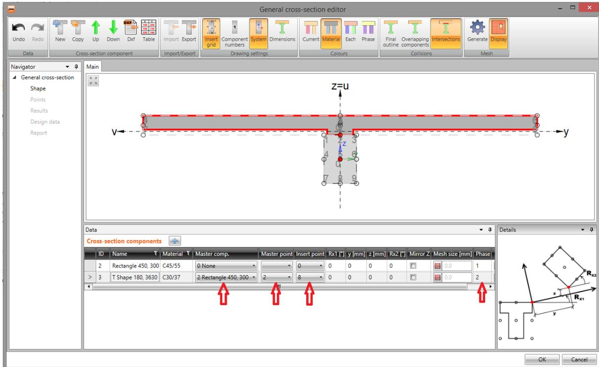
The next step is to change the position of composite slab component – to get the bottom edge of slab coincident with the top edge of the rectangular component of the first phase.
