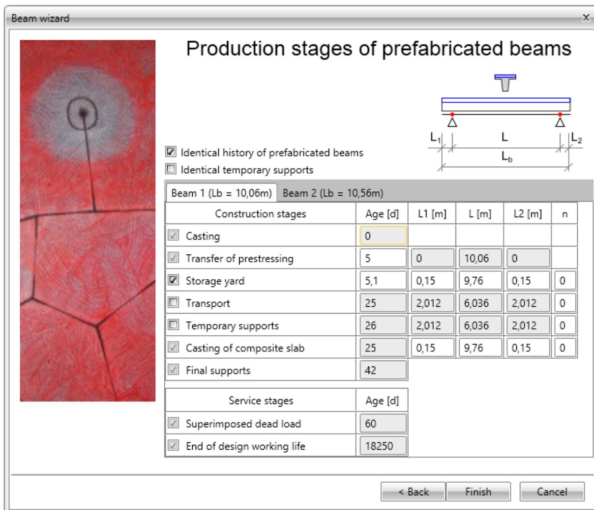
Set dialog **Production stages of prefabricated beams** as follows:
