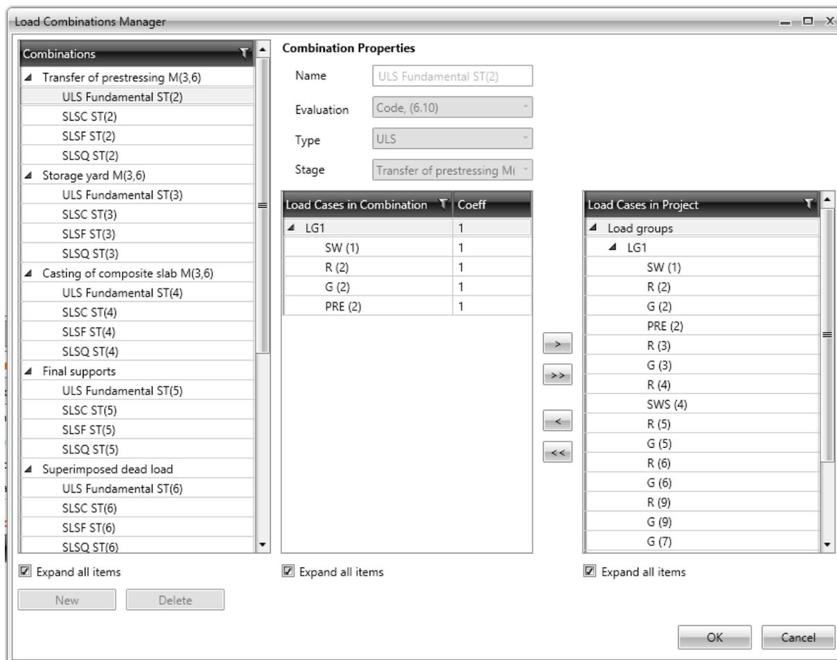
On the left, existing combinations categorized by construction stage are displayed in the tree control **Combinations**.
