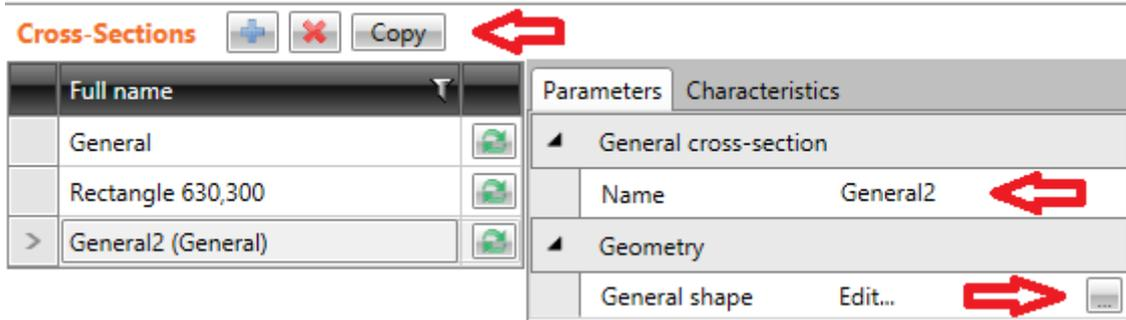
In the properties table on tab **Parameters**, rename the copied cross-section e.g. to **General2**. Click to modify the cross-section.
