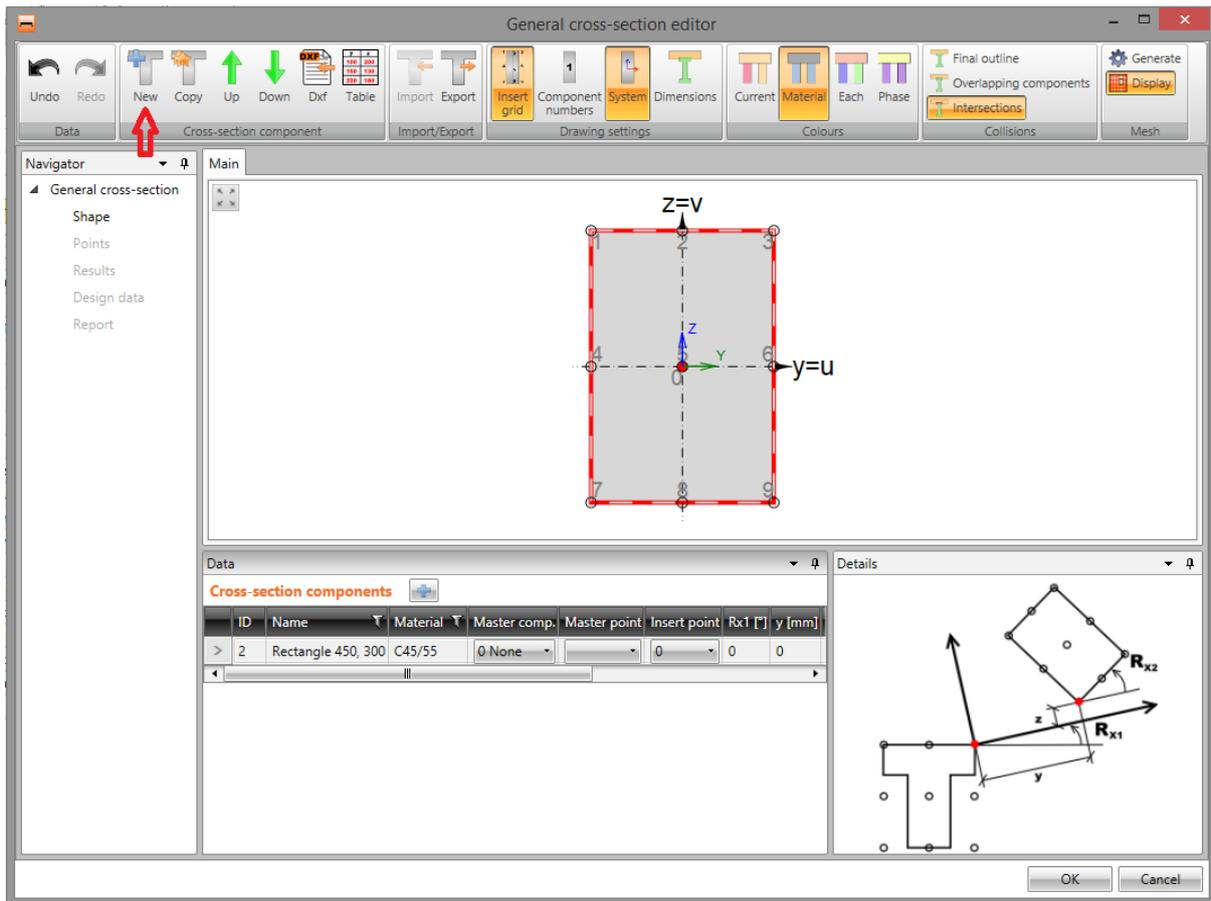
Dialog **Cross-section** navigator appears. Click picture of T-shaped section on tab **Basic** to start input of composite slab component.
