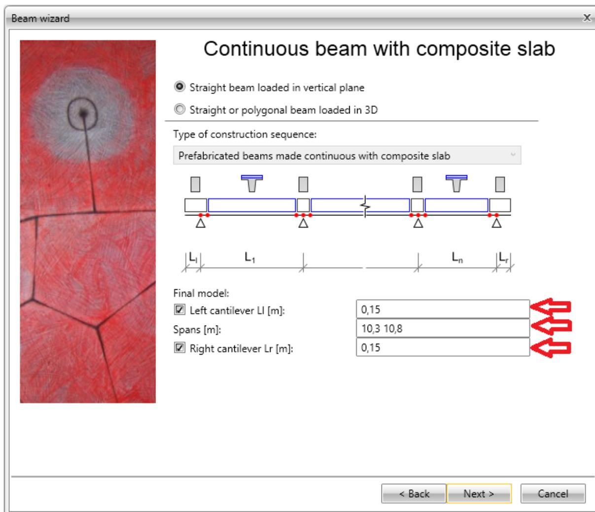
Set beam properties in the second wizard dialog **Continuous beam with composite slab** as follows:
