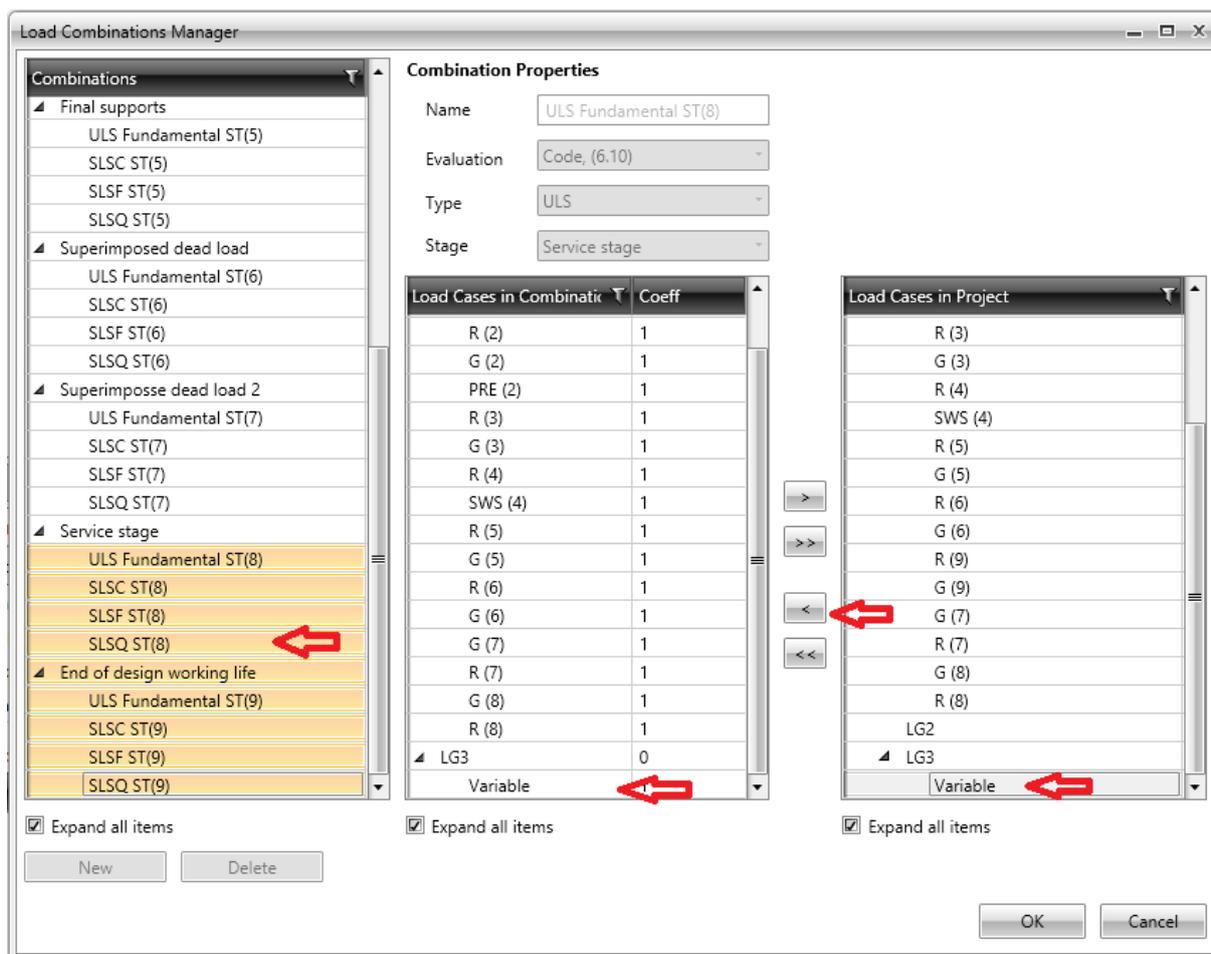
In the **Combinations** tree view, select all combinations assigned to construction stages **Service stage** and **End of working life**.
