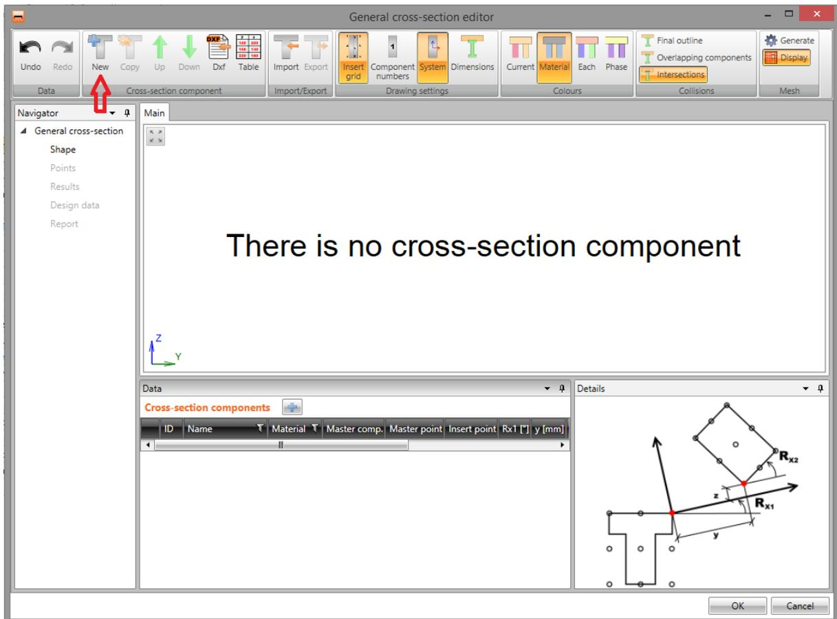
Click **New** in ribbon group **Cross-section component** to input the first component of general cross-section.
