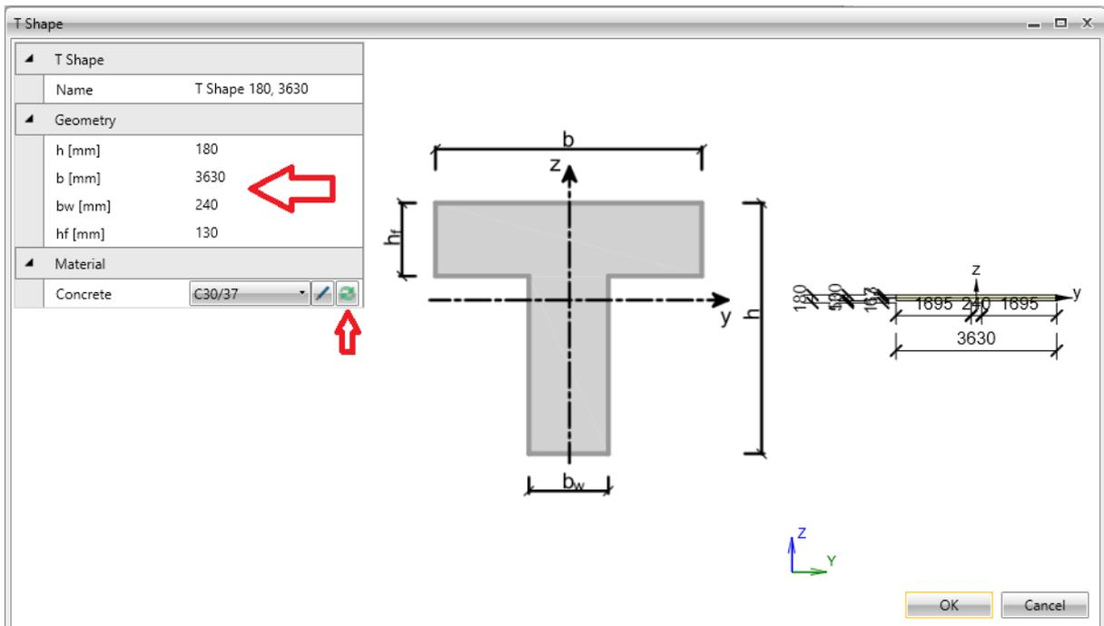
Set properties of T-shaped cross-section in **T-shape** dialog as follows:
