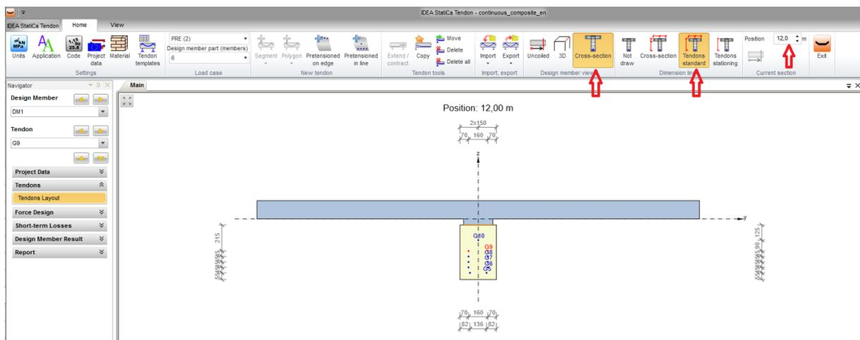
Input of pre-tensioned tendons is finished.
