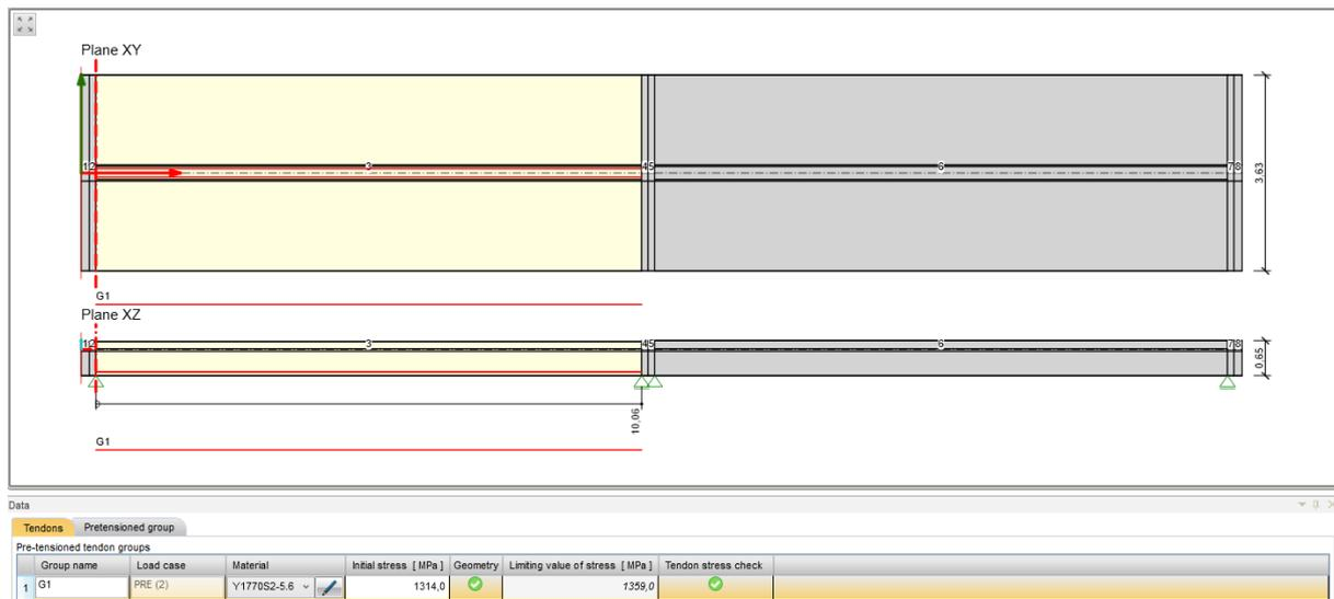
Properties of new tendon must be modified. Tendon properties table is displayed on tab **Tendons** in the **Data window**.
