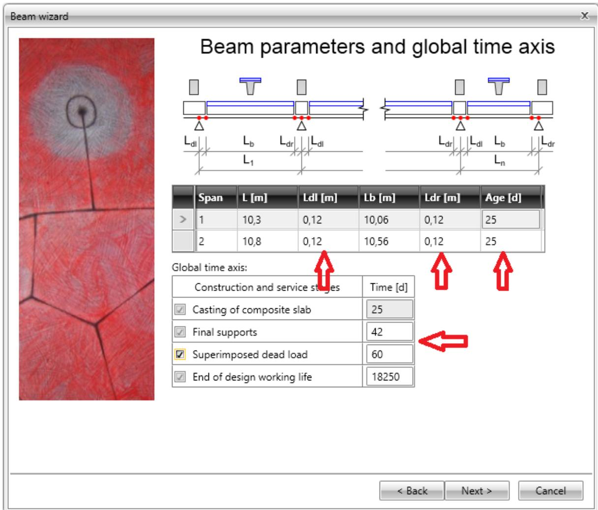
Set the table of spans properties in dialog **Beam parameters and global time axis** as follows:
