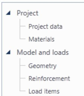
Appropriate corbel data can be input by specific navigator commands. Input of data is sorted into groups of commands **Project** and **Model and Loads**.
