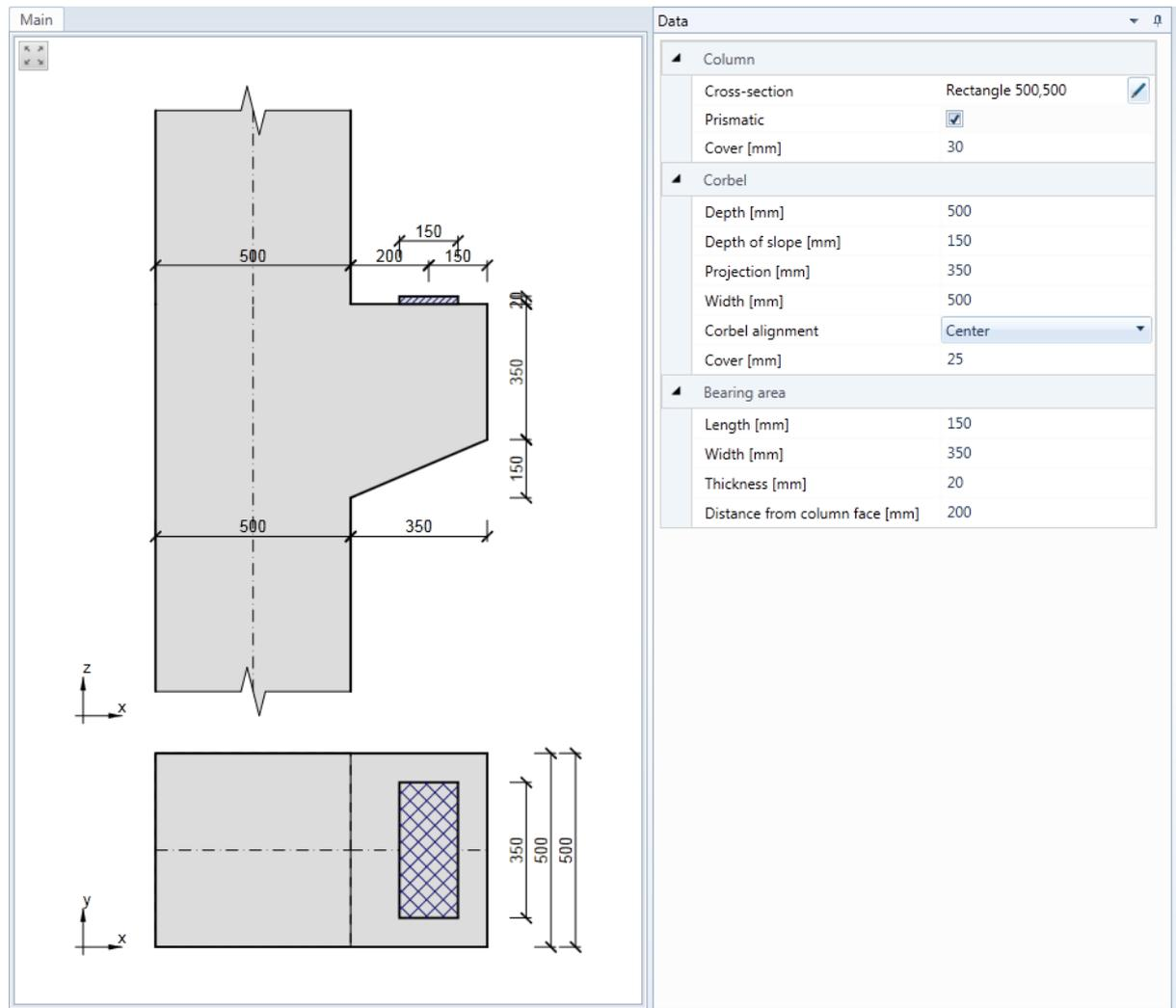
Corbel geometry is defined using properties in the Data window. Column data are defined in the **Column** properties group:
