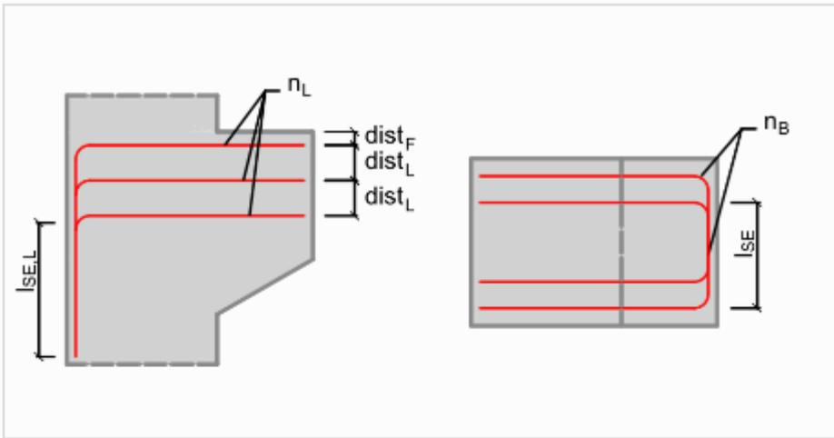
The diagram illustrates the configuration of primary plane looped bars in a corbel. The left part shows a stepped profile with two layers of bars, with parameters  $n_L$  (number of bars per layer),  $dist_F$  (distance from top to first layer),  $dist_L$  (distance between layers), and  $ISE_L$  (distance between branches). The right part shows a rectangular profile with one layer of bars, with parameters  $n_B$  (number of bars per layer) and  $ISE$  (distance between branches).
