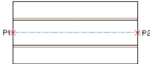
This parameter can be also specified by using the **Enter all dimensions** option. After specifying all dimensions in the dialog window, user should insert the object by indicating the insertion point (**P1**) and the rotation angle (**P2**).
