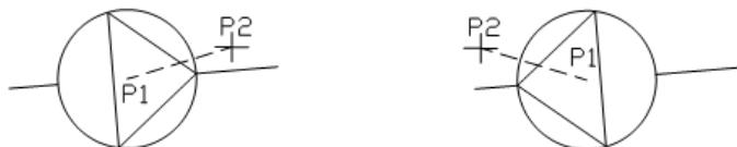
*Inserting into a line with rotation*
