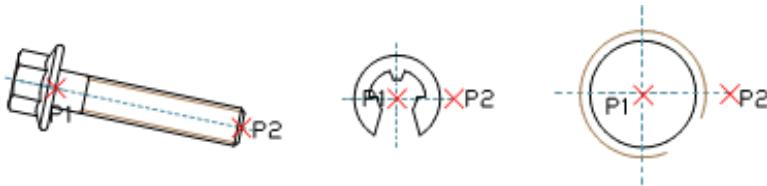
During insertion of objects such as: holes (transitional, threaded), drills, screw joints, rivets and others user should specify an additional parameter - most often the element length (e.g. the dimension that determine the hole depth or the connection thickness).
